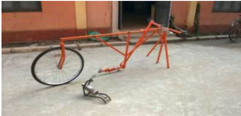
Fig: 1 Equipment for Measuring Roughness: MERLIN
